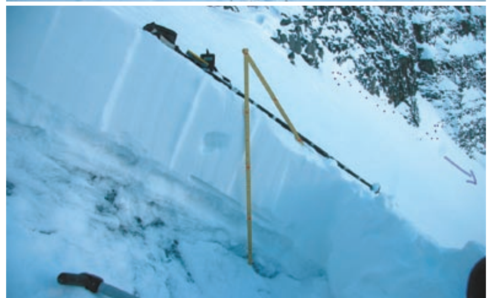
Avalanche on November 1, 2010: aerial photos show the avalanche path and location of the victims. The snow profile (above) displays the weak layer that collapsed. Photos by David George
